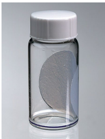
Figure 3. The filter is wetted with liquid scintillation cocktail so that it adheres to the wall of the counting vial.
