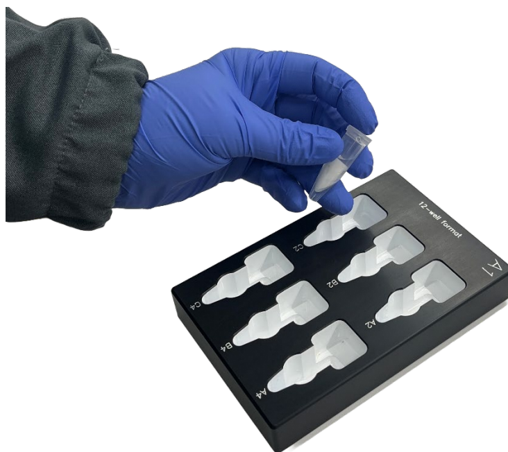
Figure 6. Wipe tests can be measured with Hidex Sense using the Hidex Eppendorf® adapter, which holds up to six samples for measurement.
