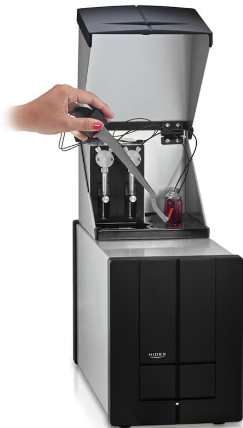
The Hidex Sense is available with digitally controlled high accuracy gas mixing system for cell viability, hypoxia and other cellular assays. Combined with wide range temperature control, advanced shaking options, bottom read, automatic aperture and focus adjustment, the Sense is always ready to use with minimal manual setup.
